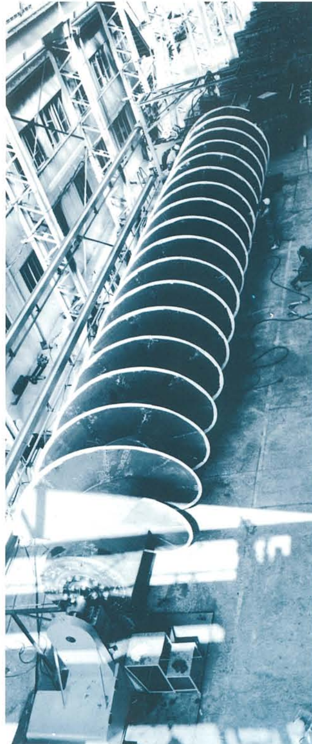
Screw Pump (screw dia: 3,000mm) under fabrication for the Arakawa 3rd Rain Water Drainage Station.
